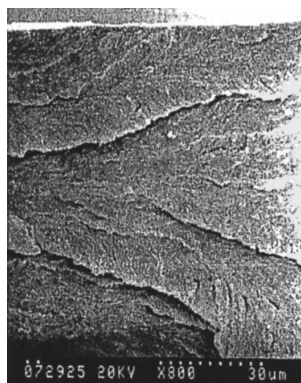
Figure 3. Scanning electron micrographs of the cross-sectional structure of the s-PTFE membrane.
